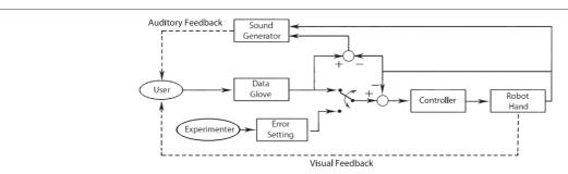
**Figure 2 Experiment setting block diagram.** The subjects controlled the robot hand's motion using a Data Glove. The different profiles of the robot hand movements were mapped to sounds and conveyed back to the subjects. During tests, the experimenter forced one of the robot hand's fingers to stop moving, which generated an error signal that was conveyed back to the subject as an auditory icon.
