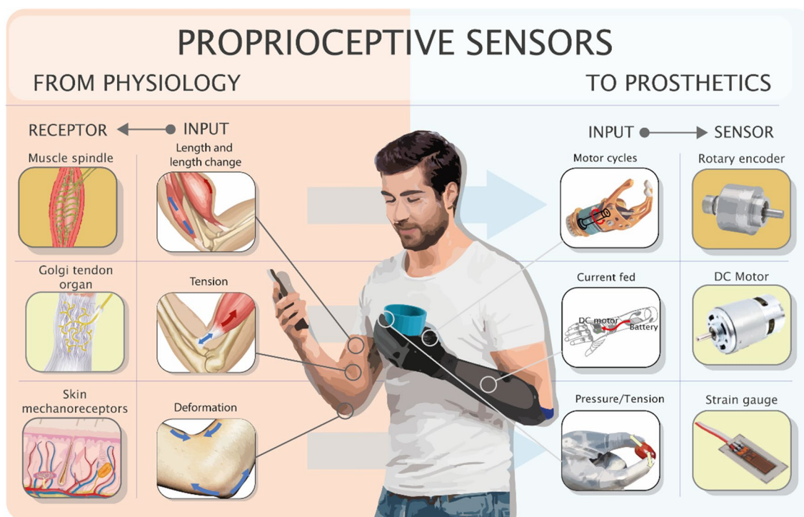
Fig. 1 Graphic comparison between physiological and artificial transduction of proprioceptive information. The outer columns show how the function of the receptors in our body (left) could be emulated by some of the common sensors already available on the market (right). In prosthetics, the employed hardware dictates the strategies to be implemented (inner columns) and the input signal may differ from the one coded by the physiological receptor. For instance, the number of cycles of the motors extracted by rotary encoders is used instead of the muscle length, while the current to the motors may replace tendon tension, as an alternative to a tension sensor, which is less common and would need to be purposefully integrated into the device additionally
