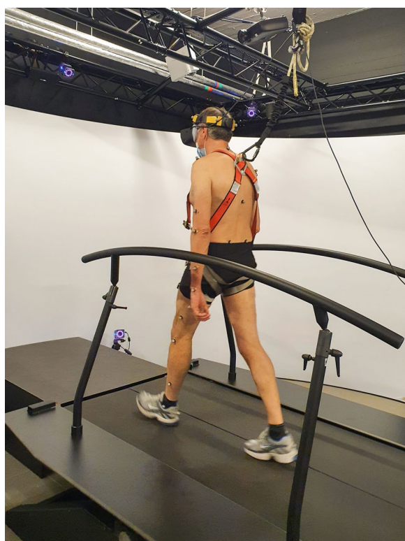
Fig. 2 A picture of a participant walking on the GRAIL system with the reflective markers while wearing the HMD
