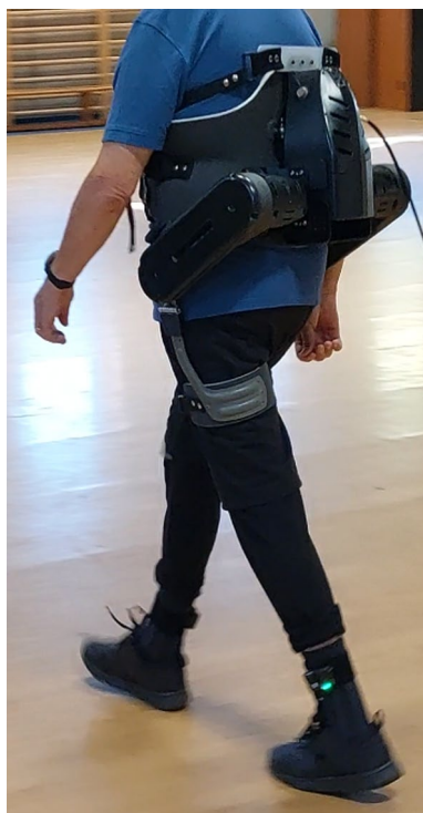
Fig. 1 The Active Pelvis Orthosis (IUVO, Pisa, Italy) worn by one of our patients
