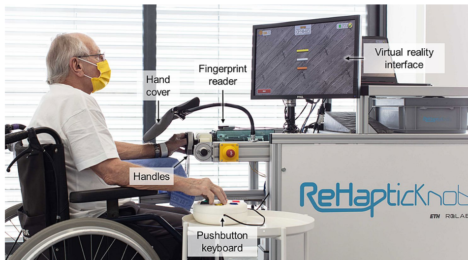
Fig. 1 Participant performing a therapy exercise with the ReHapticKnob. To train with the device, participants need to fix their fingers to the handles with Velcro straps and log in to their therapy account with the fingerprint reader. A pushbutton keyboard is used to interact with the device and the virtual environment displayed on the screen. The view of the hand (visual feedback) is blocked by the hand cover, as the exercises require users to focus on the sensory feedback from the affected hand to solve the different tasks
