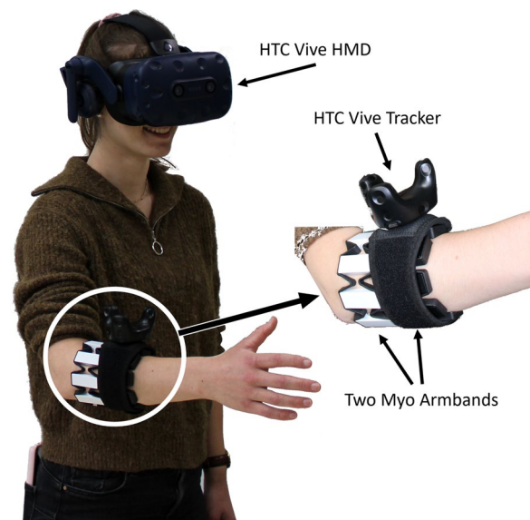
Fig. 3 Experimental setup used in the study. The figure shows a participant wearing the HTC Vive Pro head mounted display (HMD), used to visualize the virtual environment. Two Myo armbands (up to 8 sEMG sensors each) and one HTC Vive tracker are placed on the user's forearm
