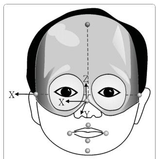
**Figure 1 Experimental setup for kinematic analysis of speech tasks.** The reflective markers were attached to the facial mask and oral areas and reference coordination system was established by marks on the mask.
