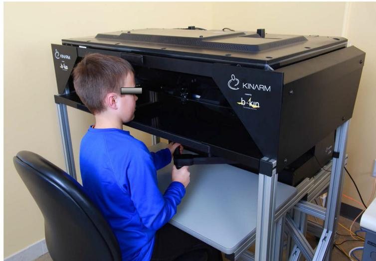
**Fig. 1** The KINARM end point robot. The virtual reality workstation projects targets onto a screen
