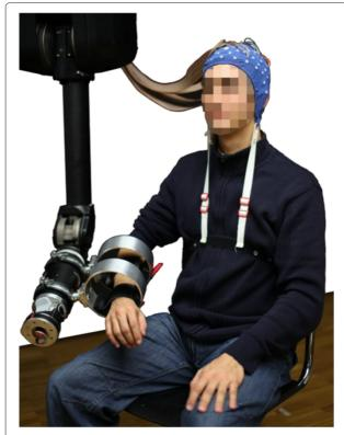
**Figure 1** Subject wearing an EEG-cap while being attached to the seven DoF Barrett WAM arm (subject consented to this image being used in this publication).
