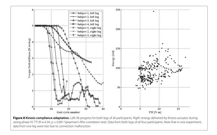
phase and the TTI, shows that a reduction in TTI reflects a significative reduction in the energy delivered by the exoskeleton (Figure 8).
