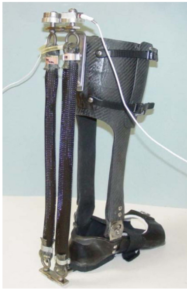
Figure 1 Subjects wore a custom fit orthosis on their left lower limb. The orthosis was hinged at the ankle to allow free sagittal plane rotation. Soleus EMG activation was recorded and processed to be used to control air pressure in the artificial pneumatic muscles proportionally. As air pressure increased, the artificial muscles started to develop tension and become shortened, allowing the powered exoskeleton to provide plantar flexor torque controlled by soleus muscle activation.
