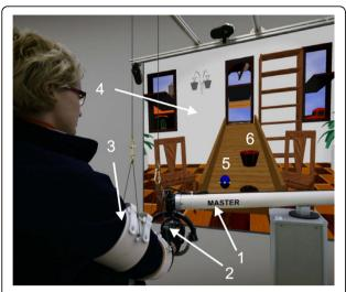
**Figure 1 Rehabilitation system**. A subject performing the virtual rehabilitation task. The subject performs the task using the robot (1) and grasping device (2) while his/her arm is gravity compensated (3). The screen (4) shows an inclined table, a ball (5) and a basket (6).
