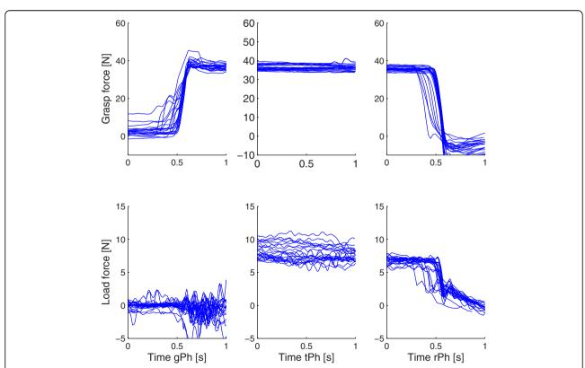
**Figure 6** The grasping force and the load force. The grasping force and the load force during pick-and-place movement for grasping phase (gPh), transport phase (tPh) and release phase (rPh). The movements were performed by a subacute subject who had no grasping assistance. Each line represents the force during single pick-and-place movement.
