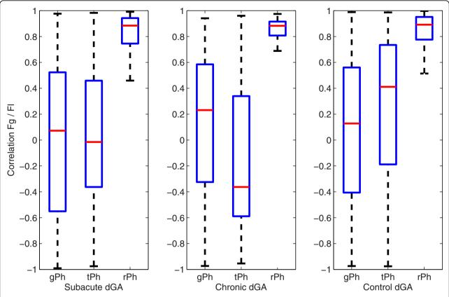
**Figure 7** The correlation between the grasping force and the load force. Correlation between the grasping force ( $F_g$ ) and the load force ( $F_h$ ) for each phase separated: grasping phase (gPh), transport phase (tPh) and release phase (rPh). The load force is the vertical component of the measured force on the end-effector. The results are shown for subacute, chronic, and control group who had no grasping assistance (dGA).
