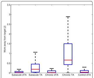
**Figure 5 Work away from the target**. Comparison of the performed work away from the target during pick-and-place movement for the subacute, chronic and control group with disabled tunnel assistance (dTA). The results of chronic and subacute group with tunnel assistance (TA) are also shown.
