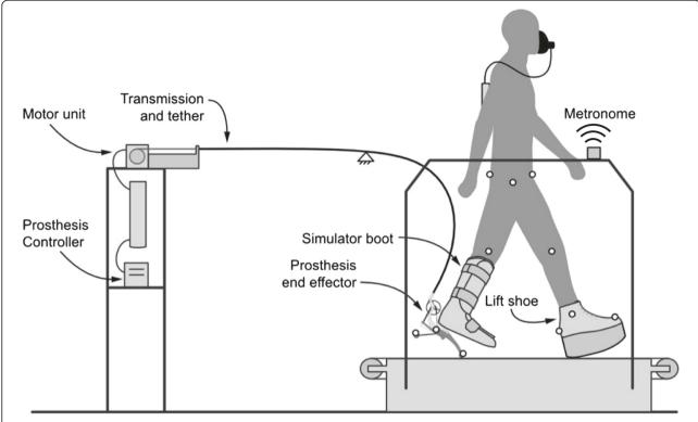
**Figure 1 Experimental setup.** Participants wore a prosthesis attached to a rigid boot and tethered to an off-board motor and control station. To compensate for the leg length difference, subjects wore a lift shoe on their other leg. Step frequency was maintained using a metronome.
