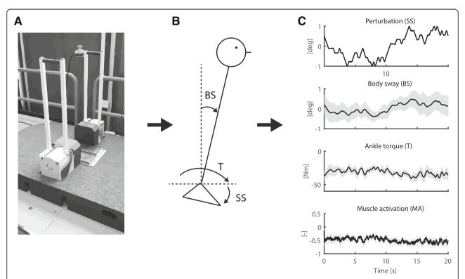
**Fig. 1** Experimental set up. **a** The Bilateral Ankle Perturbator (BAP) was used to apply the support surface (SS) rotations. **b** The actual SS rotation, body sway (BS) and ankle torque (T) were measured in combination with the muscle activation (MA). **c** A typical example of human reactions on the SS rotation. Time series are presented by mean and standard deviation averaged over data blocks
