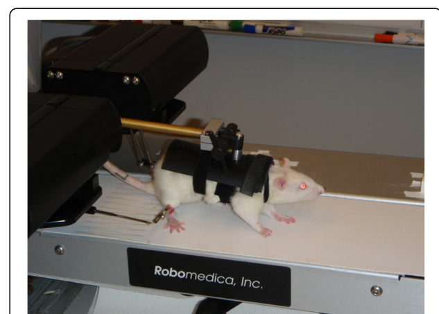
Fig. 1 BWSTT of Rats. The Rodent Robotic Motor Performance System (RRMPS) was used to track the position of the hindlimbs (ankle cuffs) as rats walked in a quadrupedal posture on the treadmill at 8 cm/s under different levels of body weight support
