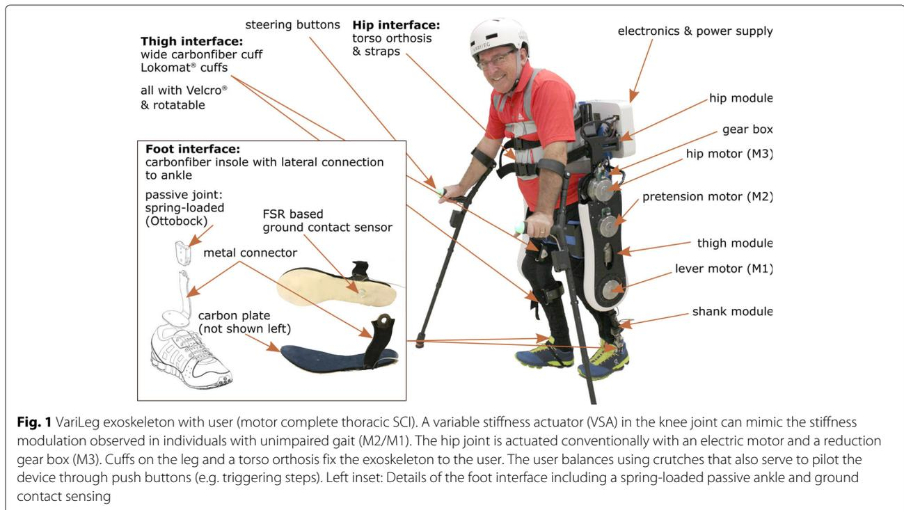
to reduce cabling complexity and to keep analog signal lines short. Covers (SLA parts made from Accura Xtreme, Müri Prototech, Switzerland) are placed outside the structure of the exoskeleton to cover sharp components and prevent any possible harm during transfer into and use of the exoskeleton.
