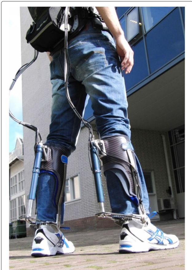
Fig. 2 The Achilles ankle-foot orthosis
