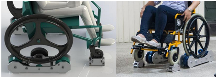
Fig. 2 Personal Wheelchair Platform. Used to support the wheelchair and provide anthropometrically correct resistance
