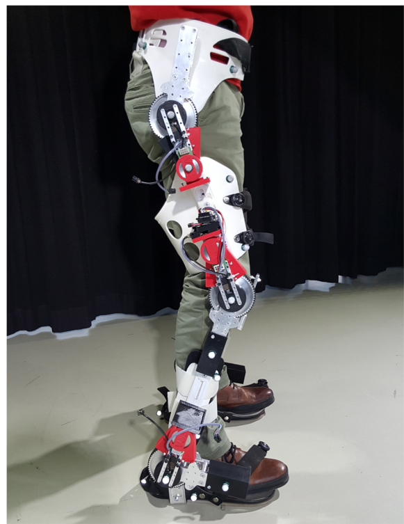
Fig. 5 The MIRAD sit-to-stand exoskeleton. A side view of the MIRAD sit-to-stand exoskeleton is shown. The power and communication cables for each joint are not present to avoid overload of the photograph. The MACCEPA actuators are placed at the hip, knee and ankle of a commercial lower limb brace
