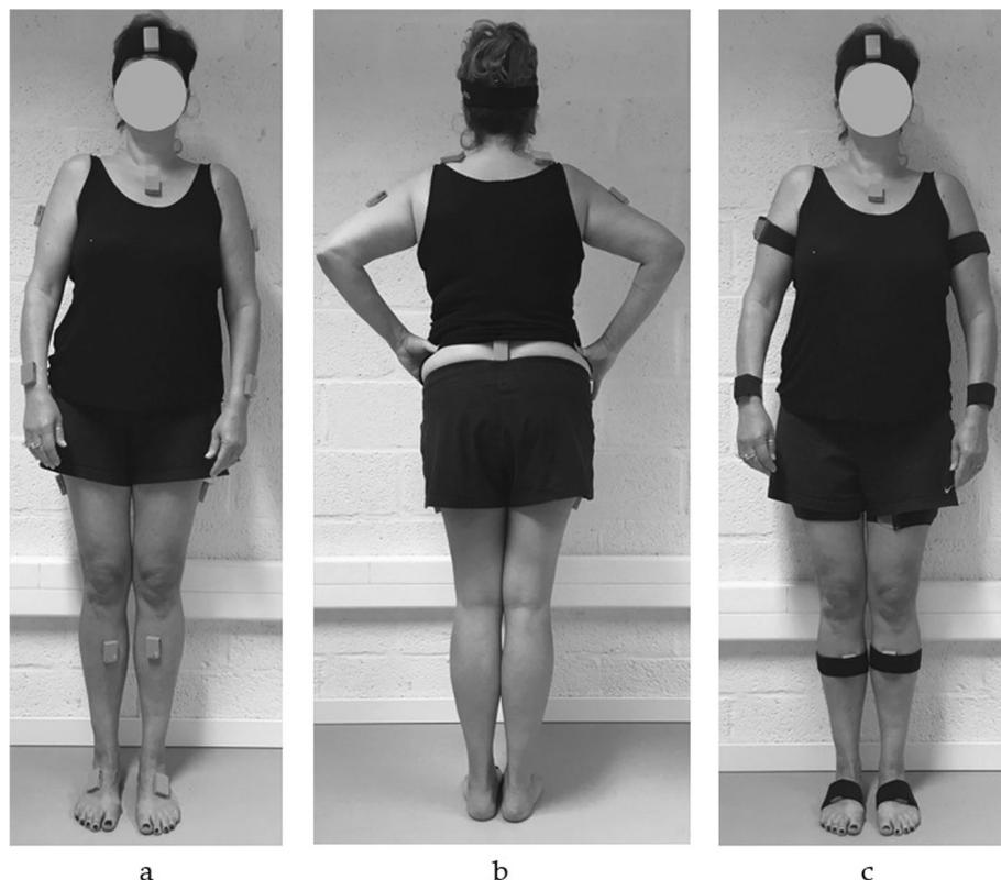
**Fig. 1** Positioning of inertial sensors in **a** anterior and **b** posterior view, and **c** anterior view with the straps to minimize soft tissue artefacts
