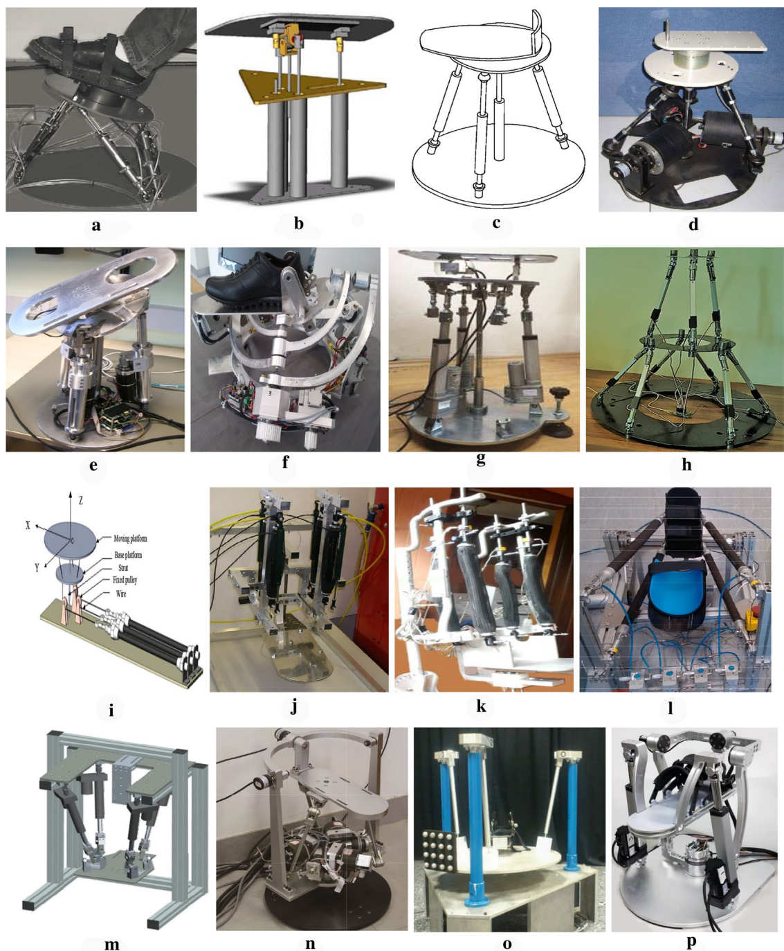
Fig. 4 PARRs with different mechanism configurations. a Rutgers Ankle -" Rutgers University"; b Reconfigurable ankle robot -" Gwangju Institute of Science and Technology"; c 3- SPS/SP mechanism -" King's College London"; d 3- RSS/S mechanism -" Heibei University of Technology"; e ARBOT -" IIT"; f PKAnkle -" Institute of Industrial Technologies and Automation"; g 2-DOFs parallel ankle robot -" Karadeniz Technical University"; h 9-DOFs hybrid PARR -" University of Birmingham"; i 2-DOFs ankle rehabilitation robot -" Wuhan University of Technology"; j Soft parallel robot (SPR) -" University of Auckland"; k Compliant ankle robot -" Nazarbayev University"; l Compliant ankle rehabilitation robot -" University of Auckland"; m Redundantly actuated ankle robot -" University of Auckland"; n 3-RUS/RRR -" Beijing Jiaotong University"; o 3- PRS -" Universidad Politécnic de Valencia"; p 2-UPS/RRR ankle rehabilitation robot -" Beijing University of Technology"
