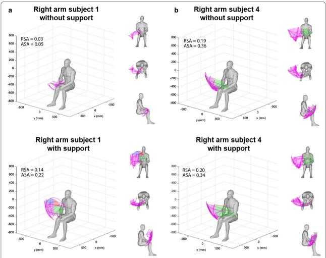
**Fig. 2** Reachable workspace with and without Yumen Arm. **a** example of subject 1, where the reachable workspace improves due to use of the Yumen Arm. **b** example of subject 4, where the reachable workspace remains unchanged when using the Yumen Arm
