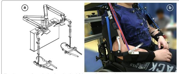
Fig. 1 Yumen arm. a Design sketch without elastic bands, b Prototype fitted on one of the participants
