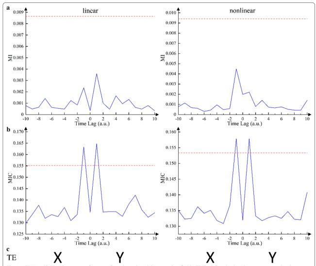
Fig. 3 a TDMI and b TDMIC curves as a function of time lag. c Causal direction identified by TE. The left and right columns correspond to the bidirectional linear and nonlinear dynamical systems, respectively. X-axis indicates delay time with arbitrary unit (a.u.). Red dotted lines are the levels of significance threshold. The data length of all models was set to 1000
