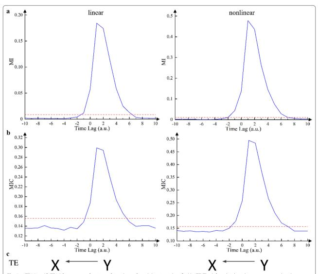
Fig. 2 a TDMI and b TDMIC curves as a function of time lag. c Causal direction identified by TE. The left and right columns correspond to the unidirectional linear and nonlinear dynamical systems, respectively. X-axis indicates delay time with arbitrary unit (a.u.). Red dotted lines are the levels of significance threshold. The data length of all models was set to 1000
