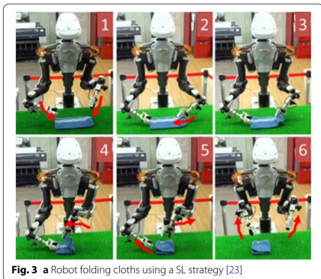
**Fig. 3** a Robot folding cloths using a SL strategy [23]
