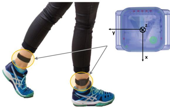
**Fig. 1** Participant wearing one inertial measurement unit attached with a flexible strap laterally above each ankle. Enlarged schematics depicts the sensor module with its local coordinate system
