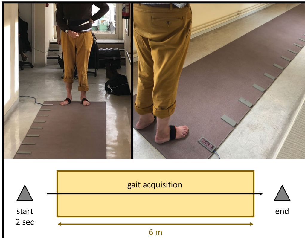
Fig. 2 Gait recording protocol. The patient is equipped with two sensors Mtw Awinda XSens ® placed on the dorsal part of each foot using Velcro bands. Walking is initiated upstream of the active surface of the GR
