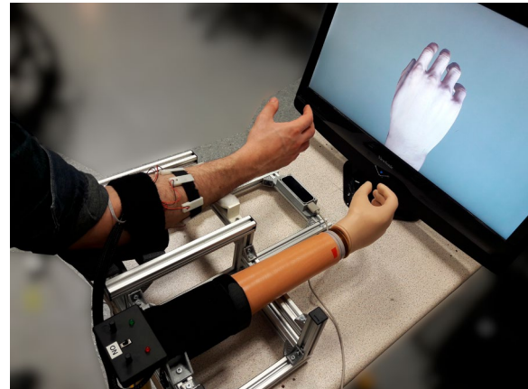
Fig. 14 Experimental setup for testing vibro-tactile proprioceptive feedback with an early version of the Smart Arm platform. [48]
