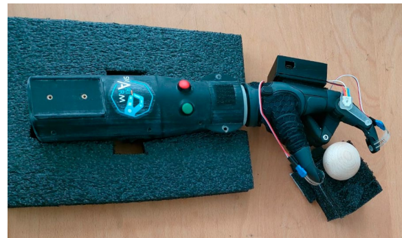
Fig. 15 Taska hand equipped with force sensors and rotary encoder [49]
