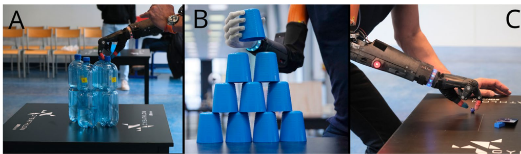
Fig. 10 Examples of tasks in Cybathlon's ARM race. A Carrying bottles (weights ranging from 100 g to 1.6 kg). B Stacking cups (photograph ©Pierre Kitmacher, Sorbonne Université). C "Clean Sweep" i.e. small object manipulation
