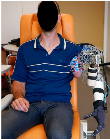
Fig. 11 Early prototype of the Smart Arm prosthesis driven with phantom limb motion [45]
