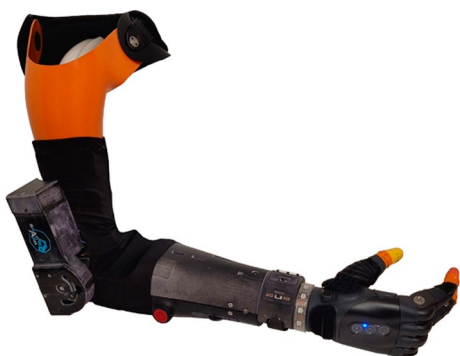
Fig. 1 The Smart ArM prosthesis in its current iteration, fitted with a Taska prosthetic hand
