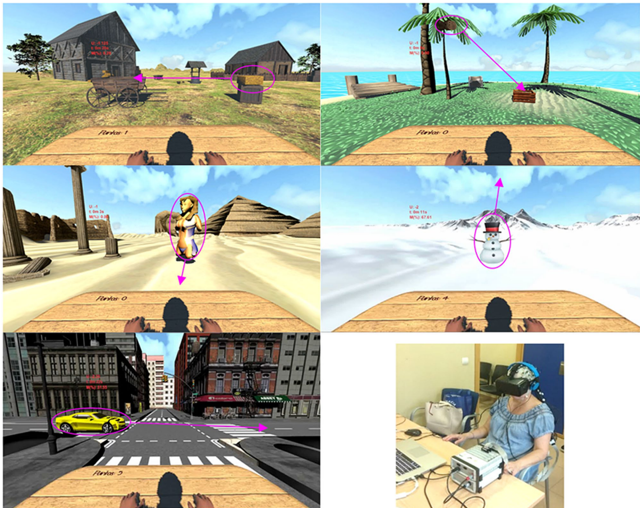
Fig. 1 Frames of the different Neurofeedback (NFB) environments designed for the intervention. Objects surrounded by the circles are the moving targets. Arrows indicated the direction and destination of the movement. Bottom right image: Experimental setup of participants, showing the Virtual Reality set up (Oculus® 3D), mounted over the 64-channel EEG cap
