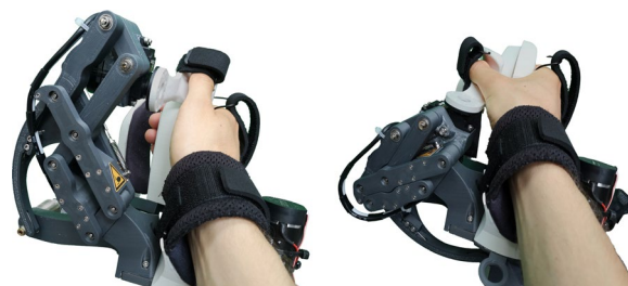
Fig. 3 Thumb circumduction movements, enabled by the remote center of motion mechanism
