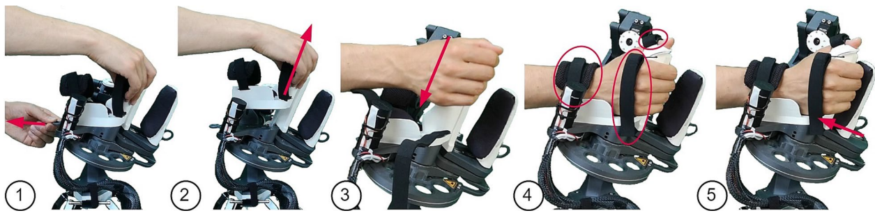
Fig. 5 Setup sequence: (1) The handle must be unlocked by pulling the lever on the back (here left side) of the hand module. (2) The handle is being removed by vertically sliding it off the hand module. (3) Once the new handle is installed, the patient’s hand can be slid onto the device without the need for finger extension. (4) The wrist, thumb and metacarpals straps are tightened with hook and loop attachments. (5) The fingertip support is tightened by sliding it towards the fingers and held in place through a ratchet mechanism
