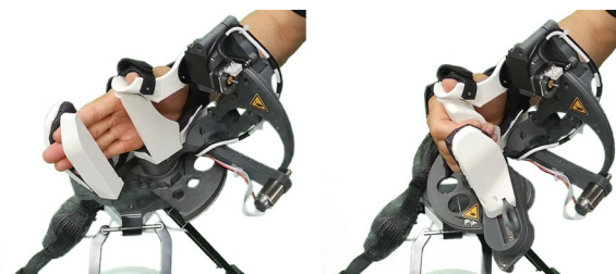
Fig. 2 Collective finger flexion and extension movements
