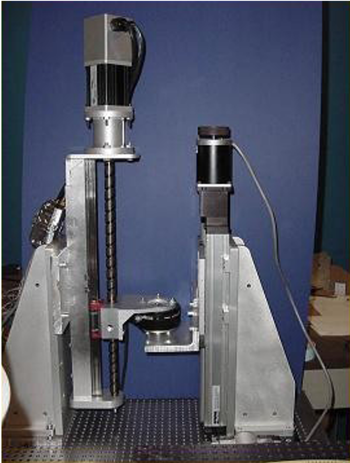
Figure 2 Constant-Velocity Friction Experiments (0.5 to 50 mm/sec). Photo shows alpha-prototype. The mean friction force was 20.075 \pm 1.056 N.
