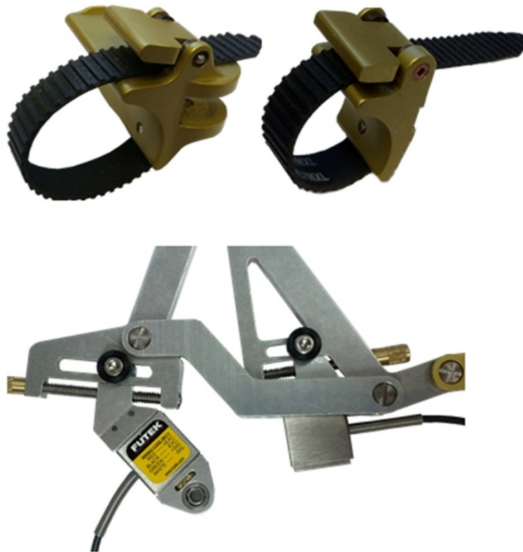
Figure 6 Finger cups with ratcheting straps for the middle phalanx (top left) and the proximal phalanx (top right) and finger length adjustment (bottom).
