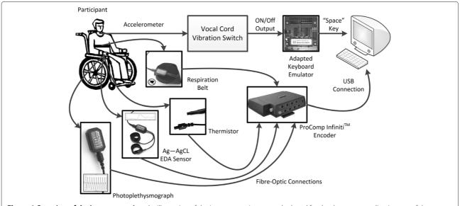
**Figure 1 Overview of the instrumentation.** An illustration of the instrumentation setup deployed for the three case studies. Images of the sensors, ProComp Infiniti encoder and the keyboard encoder were taken from the website of the the respective manufacturers.
