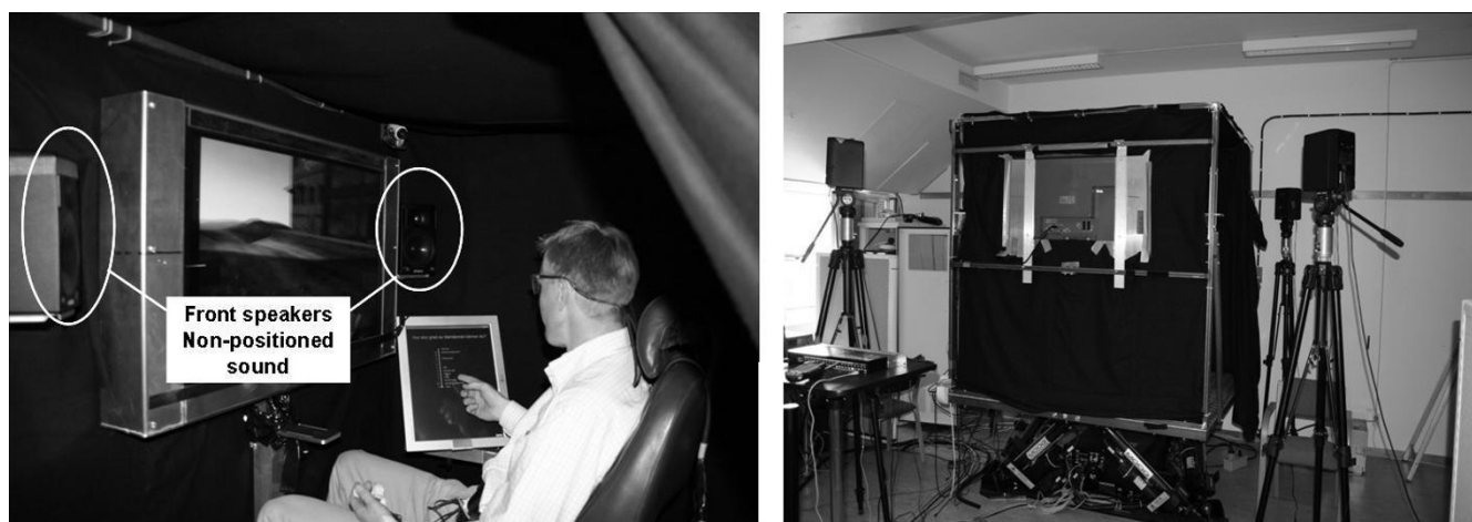
Figure 1 Picture shows front speakers location inside cabin in the non positioned sound condition (left), speakers behind the subject not visible in picture. Speakers positioned outside the cabin in the sound horizon condition (right). The right most screen displayed the Mal score questionnaire.
