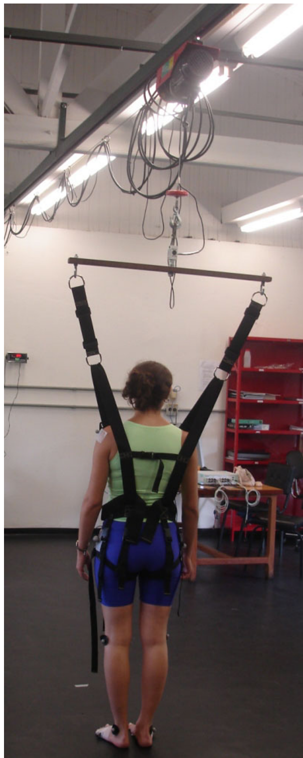
Figure 1 Partial view of the body weight support system used in the study. The rail that the electric motor slides along, the load cell, and one of the experimenters wearing the harness are shown.
