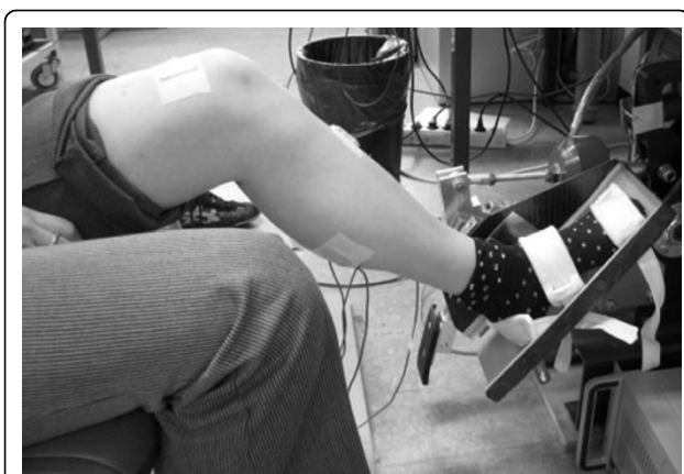
Figure 1 Measurement set-up. The subject's ankle was fixated on the footplate that was rotated by an electrically powered single axis actuator. Ankle reaction torque, ankle angle and EMG were measured during imposed ramp-and-hold movements.
