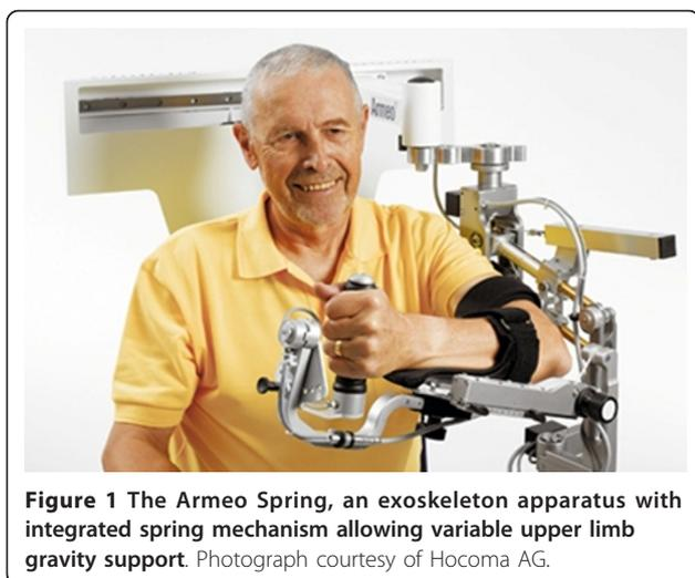
**Figure 1** The Armeo Spring, an exoskeleton apparatus with integrated spring mechanism allowing variable upper limb gravity support. Photograph courtesy of Hocoma AG.
