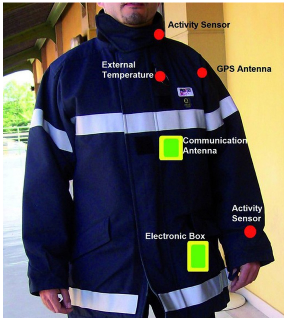
Figure 6 The ProeTEX project aims to develop smart garments for emergency responders. These smart garments integrate sensors, communication, processing and power management directly into the garment to continuously monitor emergency responders. (Courtesy of Smartex, Italy).
