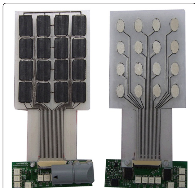
Figure 4 Multi-pad electrodes with the pressure sensor layer (left) and the universal contact layer covered with hydrogel (right).
