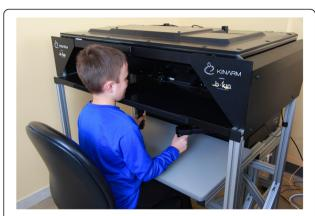
**Fig. 1** The KINARM end point robot. The virtual reality workstation makes it possible to view targets projected onto a screen
