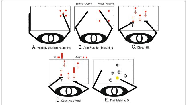
Fig. 2 The five KINARM robot tasks used in the study. a Visually guided reaching with the right arm, b Arm position matching with the right arm, c Object hit, d Object hit and avoid, and e. Trail making B (not to scale, example of the alpha-numeric alternation)
