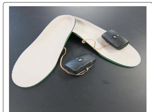
Fig. 1 Vibratory Shoe Insoles. Stochastic resonance was delivered to the soles of the feet via controlled vibratory stimuli. Vibrations were generated by piezo-electric actuators mounted within the insoles and driven by a control unit (black box) secured to the outside top of the shoe
