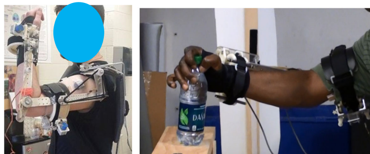
Fig. 2 SpringWear worn by subjects. Left: a subject testing SpringWear assistance on his left arm. Right: Stroke subject wearing SpringWear at his right side during functional task performance
