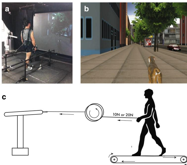
**Fig. 1** Experimental setup. (a) Virtual reality setup with HapticMaster, self-paced treadmill and virtual environment back-projected onto a screen in front of the treadmill. (b) Synchronized virtual reality scene featuring dog and city-scape. (c) Schematic of HapticMaster robotic arm, pulley, leash, and self-paced treadmill
