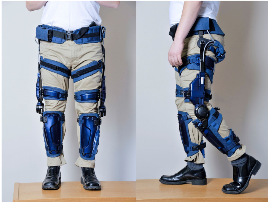
Fig. 2 Keeego™ Deroskeleton by B-Temia Inc., Quebec, Canada. The device is worn over regular clothing. Motors are located at the knees. The device is secured to the limbs with shank and thigh cuffs, and also suspended from the waist belt and chariot system that allows the hip to rotate freely
