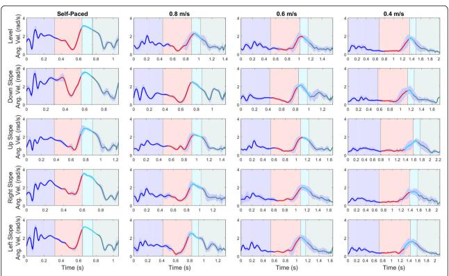
**Fig. 3** Average thigh-segment angular velocity (rad/s) and standard deviation (shaded) from a single participant for each surface condition (rows) and walking speed (columns), showing classified gait phases: Loading Response (blue), Push-Off (red), Swing (cyan), Terminal Swing (teal) for the training set. Shaded areas behind the signatures show true classes along the stride and vertical lines represent gait events
