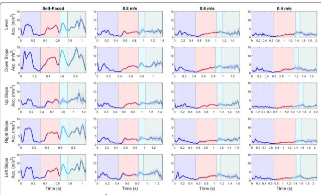
**Fig. 4** Average thigh-segment acceleration (m/s²) from a single participant for each surface condition (rows) and walking speed (columns), showing classified gait phases; Loading Response (blue), Push-Off (red), Swing (cyan), Terminal Swing (teal) for the training set. Shaded areas behind the signatures show true classes along the stride and vertical lines represent gait events
