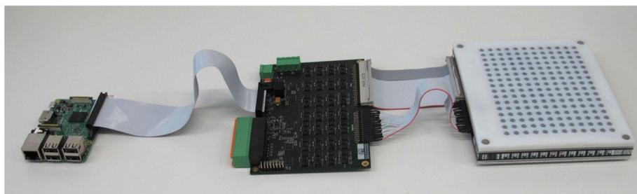
**Fig. 3** 12 × 16 BlindPAD display (right) consisting of array of 12 × 16 latching electromagnetic actuators and a 3D printed pin interface, the control board (center) and a Raspberry Pi single-board computer (left). The control board is generally mounted under the display, as in Fig. 1. All 192 pins can be reconfigured in less than 2 s. Distance between pins is 8 mm and stroke is 0.8 mm
