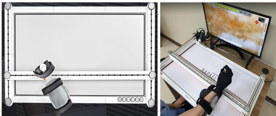
**Fig. 1** Hardware of the Smart Board. The board and forearm-supported controller. Three linear guides with an H-shape configuration enable two-dimensional planar motion of the handlebar, which is attached to the horizontal linear guide
