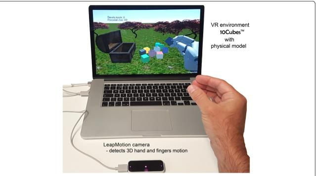
Fig. 1 10Cubes system with an infrared camera (Leap Motion Controller) for tracking of hand and finger motion was installed on the laptop computer. The LCD group used such system
