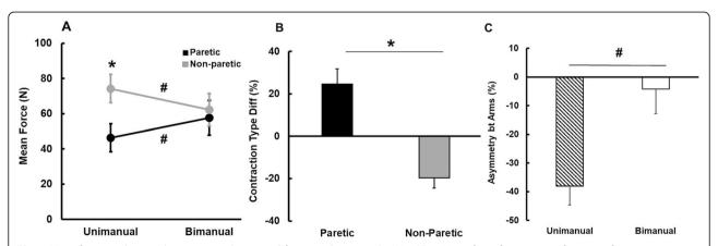
**Fig. 5** Mean force production during maximal sustained force production tasks ( $M \pm SE$ ). **a** Mean force for arms as a function of contraction types, **b** Contraction type difference of mean force, and **c** Asymmetry between arms of mean force. *Asterisk* (\*) denotes significant difference (P < 0.05) between paretic and non-paretic arms. *Number sign* (#) indicates significant difference (P < 0.05) between unimanual and bimanual conditions
