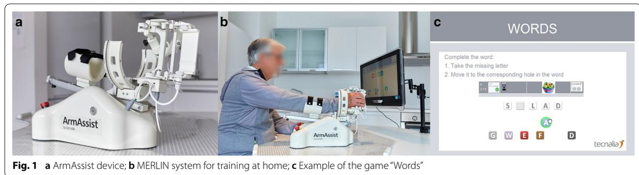
**Fig. 1** a ArmAssist device; b MERLIN system for training at home; c Example of the game “Words”
