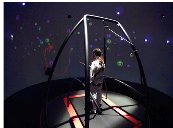
Fig. 1 The CAREN High End (Motek Medical, The Netherlands) has a 6-degree of freedom (three translation axes, three rotation axes) moveable platform that is synchronized with a virtual visual scene projected on a 360° dome-shaped screen (projection resolution 1920X1080 lines). A split-belt treadmill is embedded in the platform (not operated in this study). A motion capture system (Vicon) and a pair of force plates embedded in the treadmill provide data on the participant's spatiotemporal position during the task (sampling rate 120 Hz). The participant who performs the DOME-CTT VR adaptation (see text), is secured with safety harness, holding a wand-like pointing stick with a marker on its edge in order to control the avataric red ball and to move it towards the target ball
